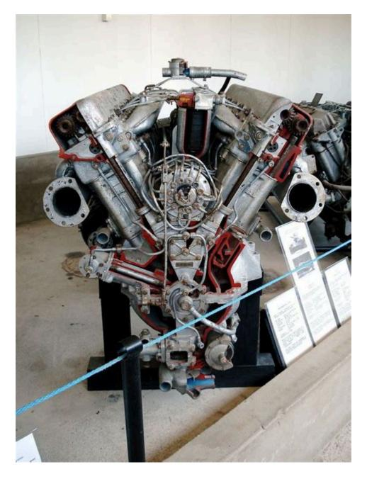
The Kharkiv model V-2 was a Soviet diesel tank V-12 engine, the V angle at 60°, with dual overhead camshafts per bank, four valves per cylinder opened by bucket-style followers and direct fuel injection, features found on modern high-performance diesel engines. Designed at the Kharkiv Locomotive Factory by Konstantin Chelpan and his team, it is found in the BT-7M, T-34, KV, IS and IS-10.
