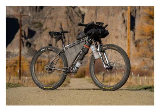
Why Cycles / El Jefe. 2021 Why Cycles El Jefe Base. 2021. 2021. Base. Category Hardtail Cross-country MTB. Design Flat Bar, Hardtail (Front suspension) Frame Titanium. Suspension 120 mm fork travel. Features Disc brake, Single-speed capable. Small size 4 sizes (Small to XL) size XL. Small.
