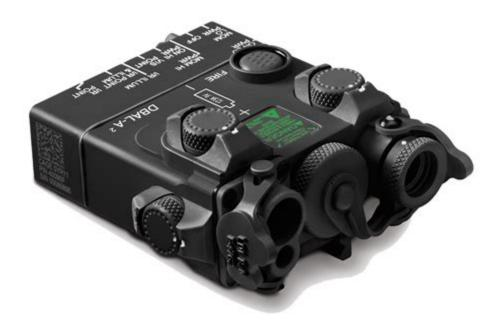
Page 13: Equipment Description. CHAPTER 2- - E QUIPMENT DESCRIPTION 2. 1 SYSTEM DESCRIPTION The DBAL-I is a Class IIIa laser device that features an IR POINT and IR ILLUM for use with a NVD. The IR beams can be operated individually or in combina- tion, in both low power (LO PWR) and high power (HI PWR) settings.
